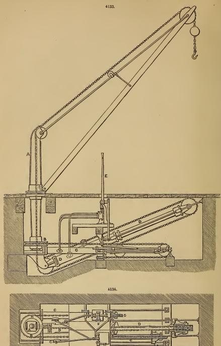
P has access to both sides of the piston, and the lower power is then obtained ; while for the higher power the valve C is closed, and the exhaust-valve D is opened, whereby the front side of the piston is kept constantly open to the exhaust E. In cases where three powers are required, three
